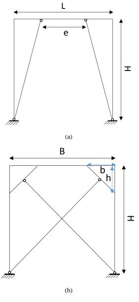
Fig. 1: Sample frame: (a) EBF, and (b) Knee braced frame.
