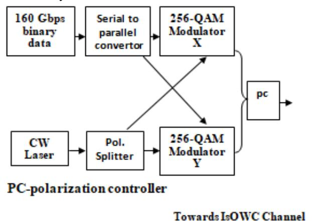
Figure 1. (b) Representation of internal structure of PDM-256-QAM
