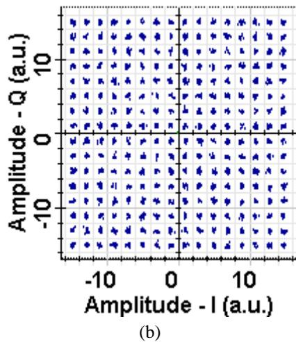
Figure 3. Constellation diagram of PDM-256-QAM for Polarization X (a) at 2000 km (b) 22,000 km
