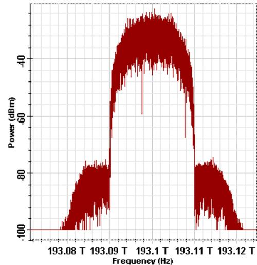
Figure 2. Optical carrier spectrum of PDM-256-QAM
