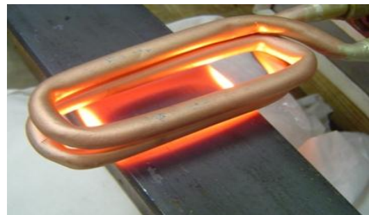
Fig. 6 Induction heating equipment
