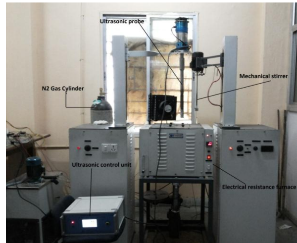
Fig.2 Ultrasonic assisted Stir Casting set up
