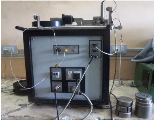
Fig. 3 Pin-on-disc type wear testing machine
