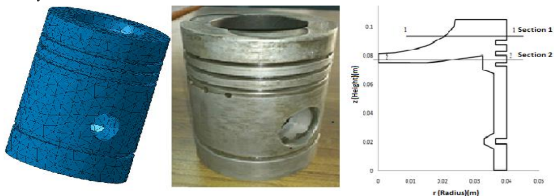
Fig.1 FE discrete model, actual and 2-D cut view of the piston model
