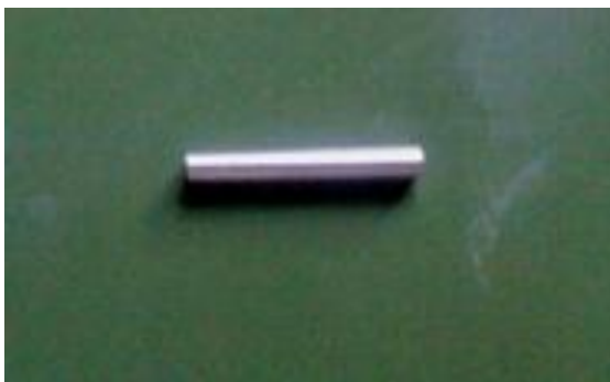
Fig. 1 Raw material (SS 316 grade)
