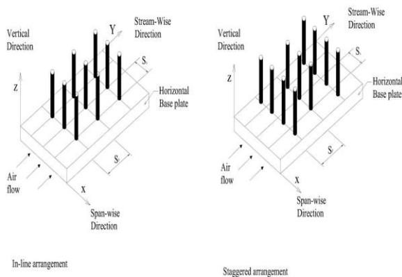
Fig. 2. Pin-fin assembly (a) Inline (b) Staggered
