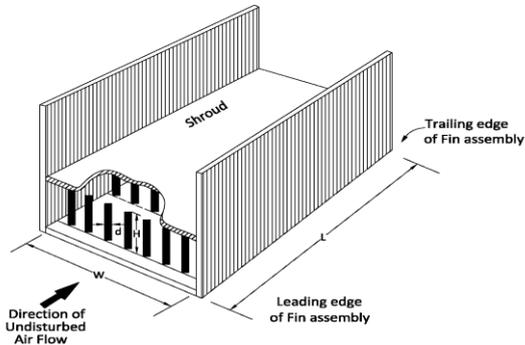
Fig. 1. Ensemble of pin fin with shroud
