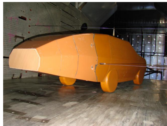
Figure 6.1: A modified vehicle model having installed a rear fairing
