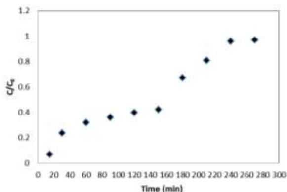
Fig.4 Breakthrough point for Nickel (II) Biosorption
