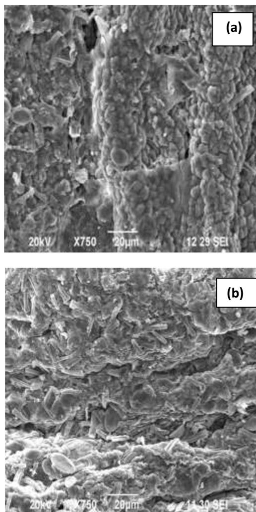
Fig.1. SEM images of *S.swartzii* (a) before Ni (II) biosorption and (b) after Ni (II) biosorption.
