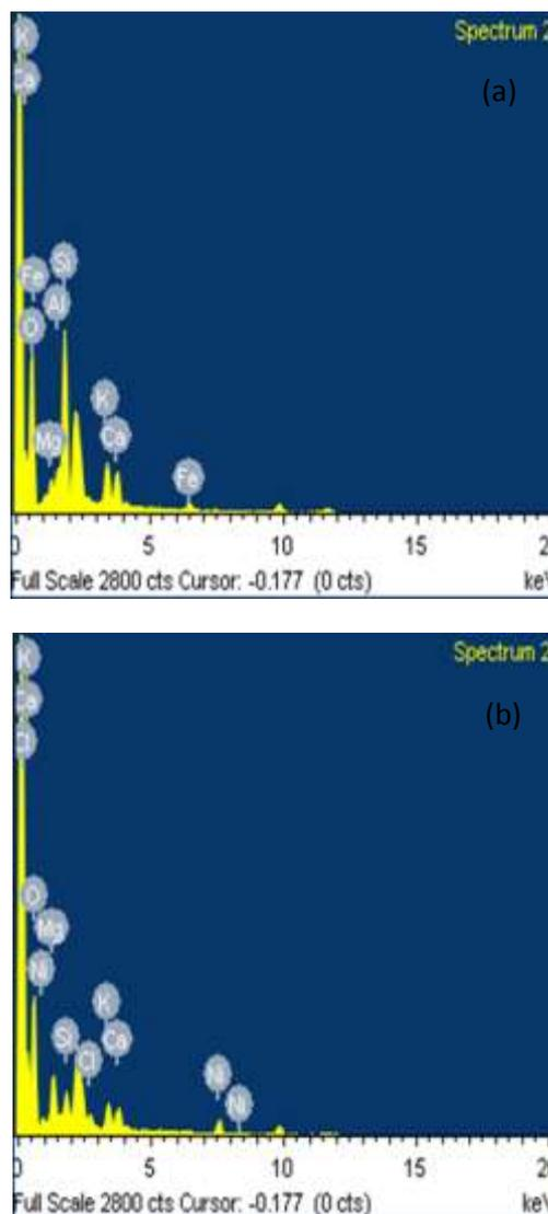
Fig. 3. EDAX analysis of *S. swartzii* (a) before Ni (II) biosorption and (b) after Ni (II) biosorption
