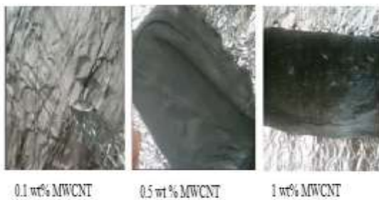
Fig2.Fiber mats which is collected from electrospinning unit
