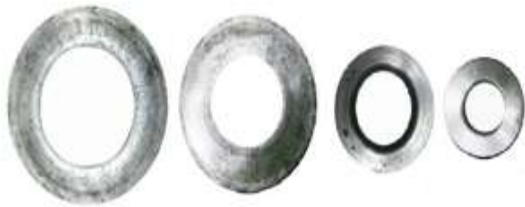
Fig.15 Machined Dies for Multi-stage Deep drawing process
