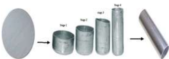
Fig.17 Conversion of Aluminium blank to tube
