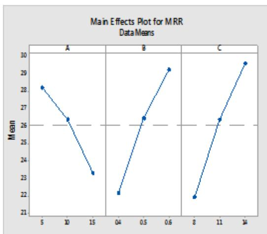
Fig. 5 Main effects plot for the Material Removal Rate
