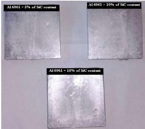
Fig. 2 Prepared specimens
