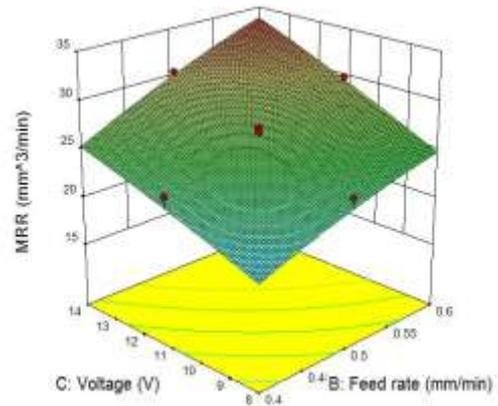
Fig. 8 Response surface graph due to interaction of Feed rate and voltage on material removal rate
