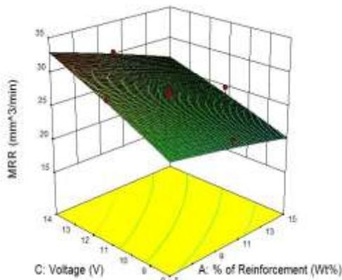
Fig. 7 Response surface graph due to interaction of percentage of reinforcement and voltage on material removal rate
