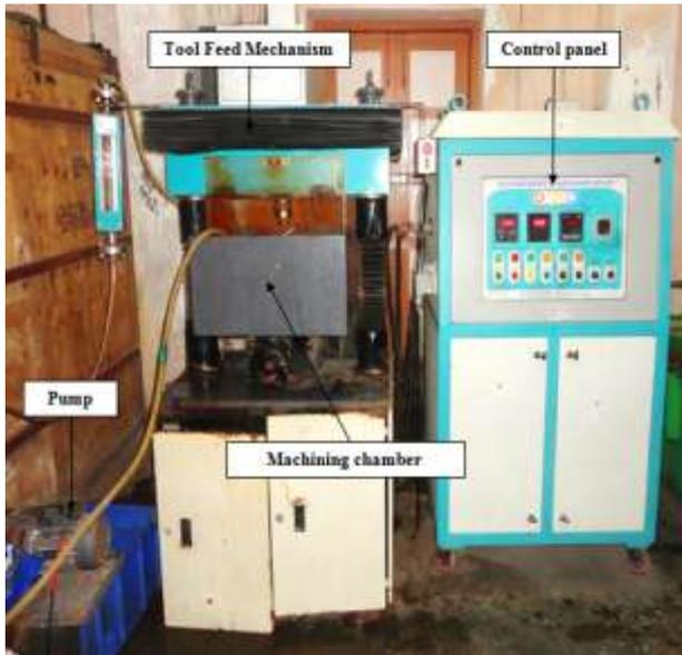
Fig. 3 Electro-chemical machining set up
