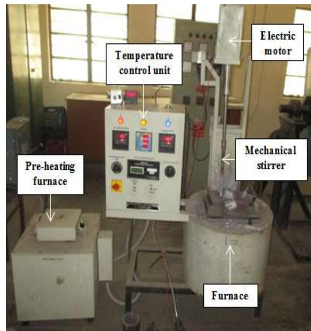
Fig. 1 Stir casting set up
