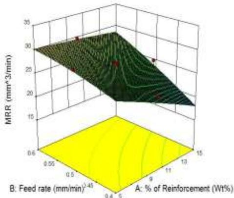
Fig. 6 Response surface graph due to interaction of percentage of reinforcement and Feed rate on material removal rate
