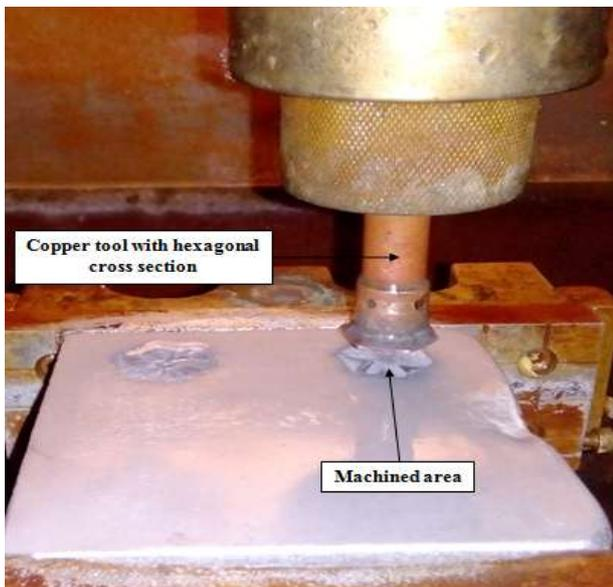
Fig. 4 Copper tool with hexagonal cross section
