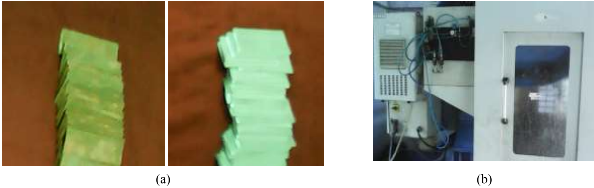
Fig. 2 (a) Base materials, (b) FSSW equipment
