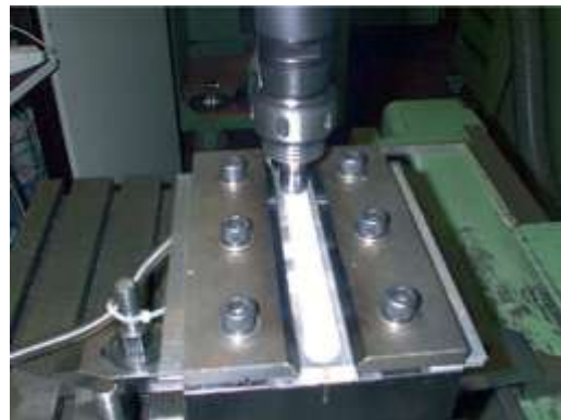
Fig.1 Photograph of the welding process and weld bead appearance
