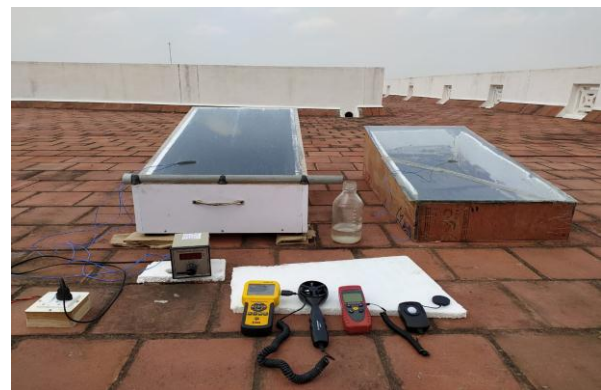
Fig. 4 Photographic view of Single basin single slope solar still
