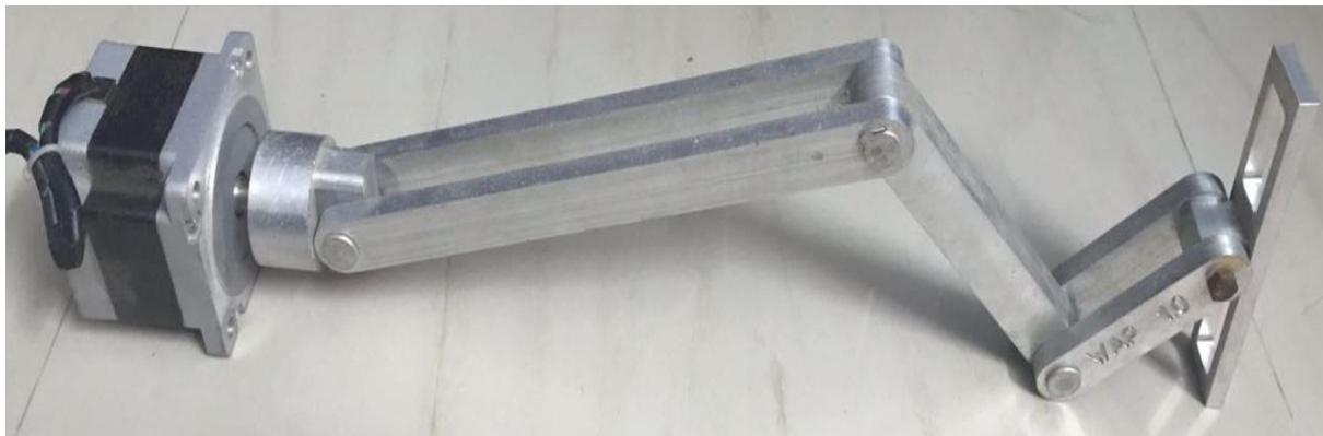
Fig. 3 Links attached with one another with aluminum rivet
