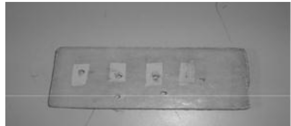
Figure 3: Drilled 8 mm GFRP plate
