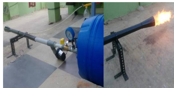
Fig. 2 Prototype model of scram jet engine before and after Combustion
