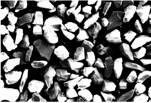
Fig. 3 SEM image of erodent alumina (Al 2 O 3 )
