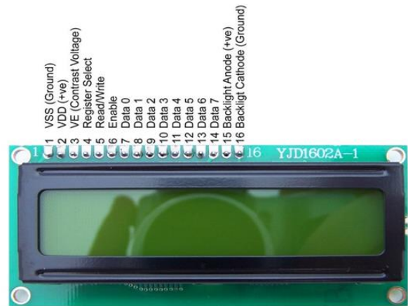
Fig. 4 LCD PIN Details
