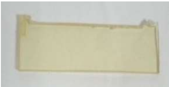
Fig. 1 Prepared sample of neat epoxy
