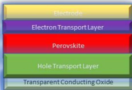
Fig. 12 Schematic illustration of the p-i-n structure
