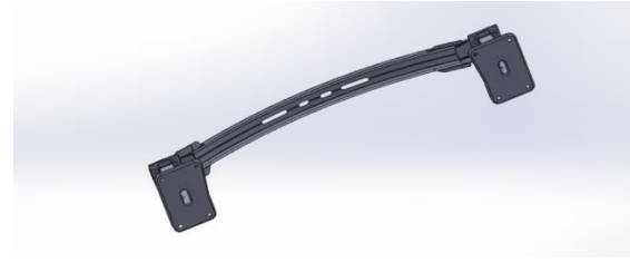
Fig. 1 CAD model of original bumper beam
