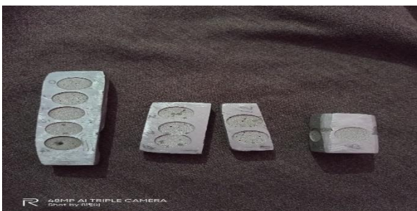
Fig 11. Machined Al/Al 2 O 3 composites.
