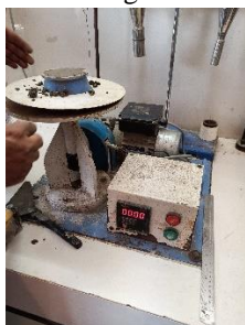
Figure 6. Flow table testing Figure 7. Mortar mixer
