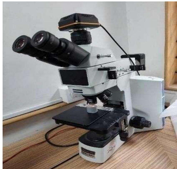
Fig 5: High – Resolution microscope for Coating thickness measurement
