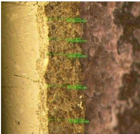
4.2 Coating thickness measurement results
