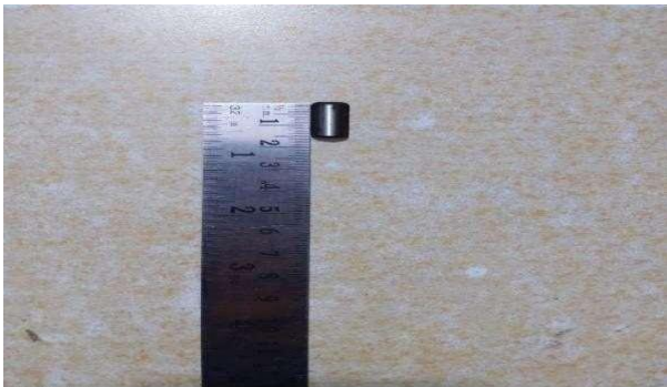
Fig 3: Wire cut sample (4x15mm)
