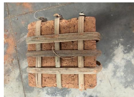
Fig 7 :- Model rammed earthen wallet retrofitted using bamboo strip in both ways
