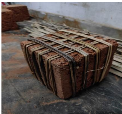
Fig 9 :- Model rammed earthen wallet retrofitted using banana petiole strip in both ways
