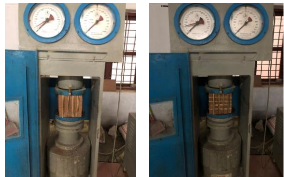
Fig 11 :- Testing of rammed earthen wallet retrofitted using banana petiole strip in one and both ways.
