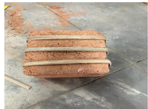
Fig 6 :- Model rammed earthen wallet retrofitted using bamboo strip in one way
