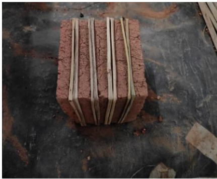
Fig 8 :- Model rammed earthen wallet retrofitted using banana petiole strip in one ways
