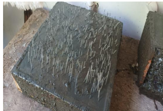
Fig 3: Mould with POF after pouring concrete in cube and panel
