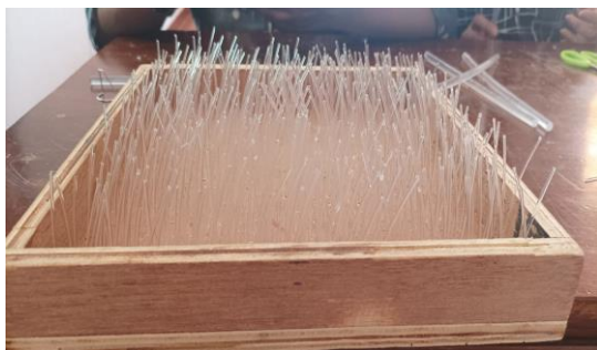
Fig 2: The formwork for panel mould.
