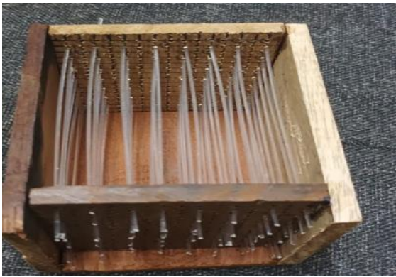
Fig 1: The formwork for cubic mould.
