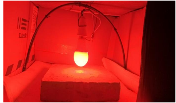
Fig 6: Artificial light transmittance experimental setup
