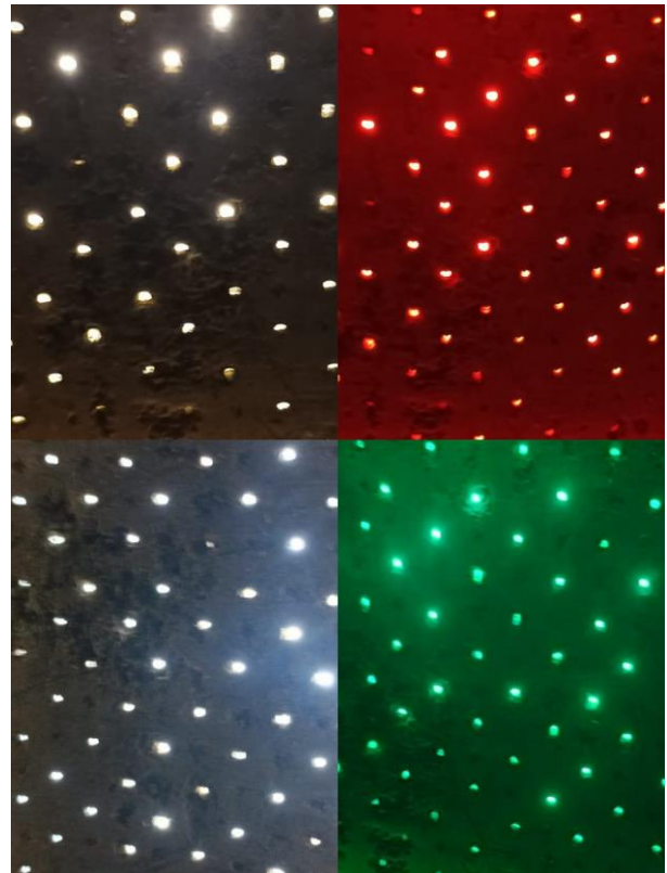
Fig 10 :Light transmitting concrete panels by using different colour LEDs.
