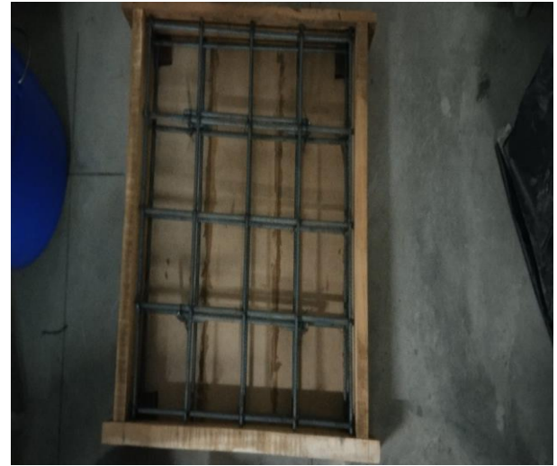
Fig 6: Slab mould with reinforcement
