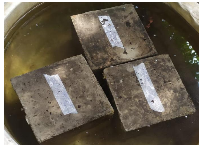
Fig 4 curing under acidic environment
