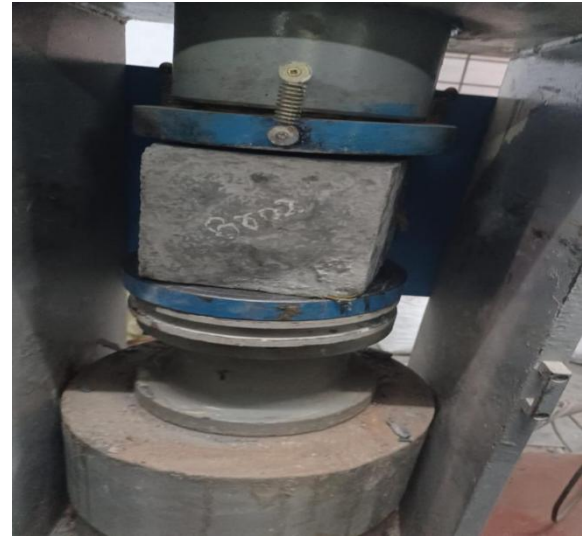
Fig.3 cube specimen at compressive testing
