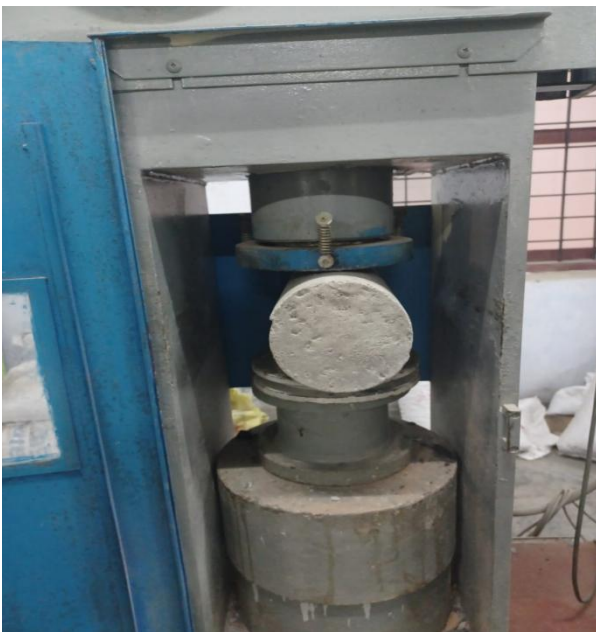
Fig 4 Specimen for split tensile test
