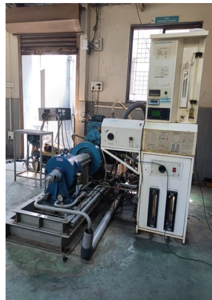
Fig 1- Pictorial view of Experimental Setup-Common Rail Direct Injection Research Diesel Engine.
