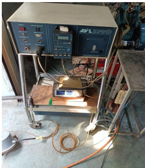
Fig 2- Setup of AVL 444 Digas Analyser with AVL 437 Smokemeter.
