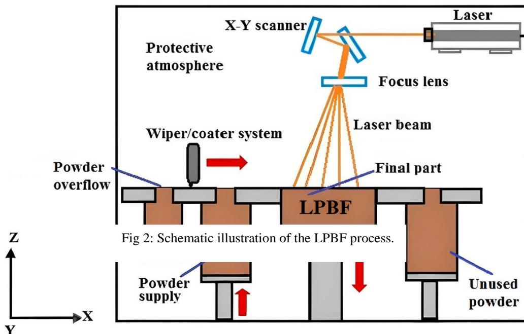
Fig 2: Schematic illustration of the LPBF process.
