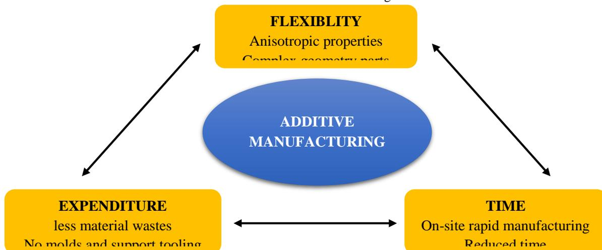
materials (FGM) for structural components in AM is time, cost, and flexibility advantages (Fig 2).
